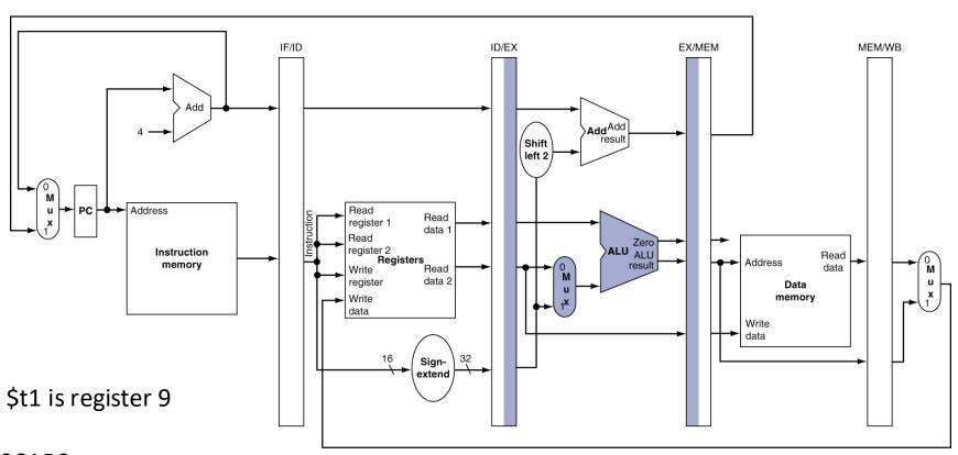
\$t0 is register 8, \$t1 is register 9 \$t0 holds 5 \$t1 holds 0x4810CAB0 0x4810CAB0 holds 12
